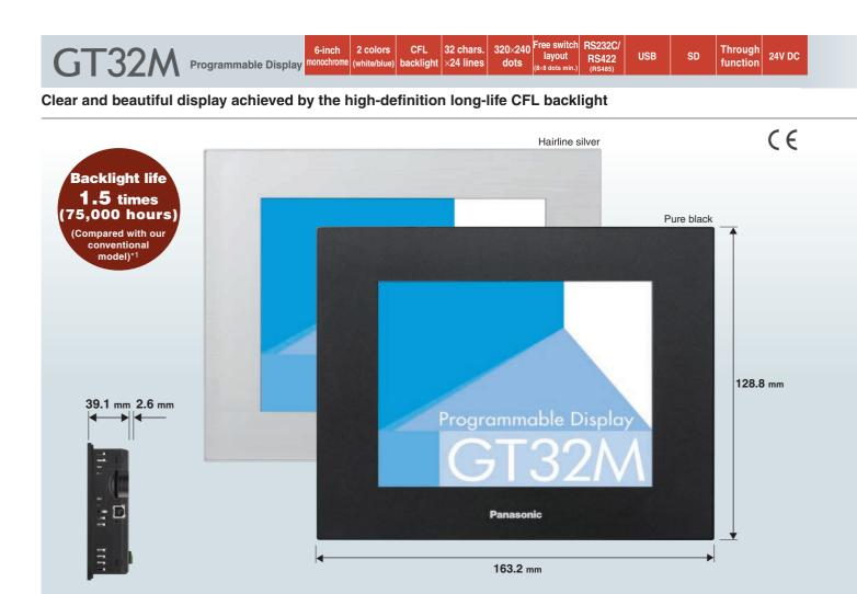
The industry's smallest size in the 5-inch class, and 39.1-mm thin and cool body design (GT32M/GT32T)
